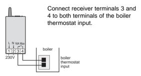
If necessary, remove the shunt (electric wire) connecting the two
