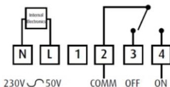
Switch live from programmer or mains feed from wiring centre (fused 3 Amp)
