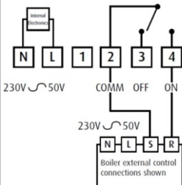
This diagram shows a typical receiver and combination boiler installation, where the external boiler control is connected via switching terminals (a link may have to be removed on the boiler switching control terminals). Mains supplies to both the receiver and the boiler are omitted for clarity. Please consult the boiler manufacturers installation handbook before commencing any installation work.
