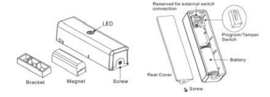
3. Use the screws or adhesive tape to fix the cover on the frame along the opening edge of the door or window. See figure below.
