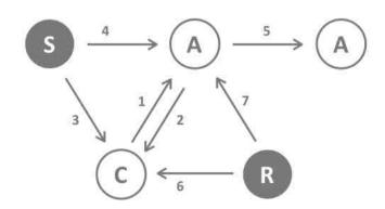
There are two different role a controller can have. There is always one single primary controller that is managing the network and including/excluding devices. The controller may have other functions - like control buttons - as well. All other controllers don't manage the network itself but can control other devices. They are called secondary controllers. The image also shows that its not possible to operate a sensor just from a remote control. Sensors only communicate with static controllers.
